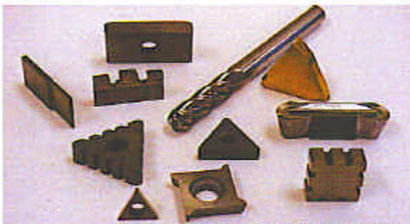
A selection of cutting tools made from polycrystalline tungsten carbide, which has no binder, as shown in the micrograph (inset).
